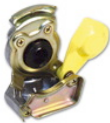
095.004 452 200 212 0 (81.51220.6025) Automatic Coupling, Yellow M22x1.5
